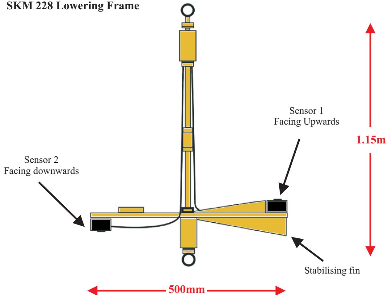
The lowering frame enables Skye light sensors to be mounted vertically (facing upwards and / or downwards) suitable for underwater measurements. Each Skye sensor is fully cosine corrected and accepts light from a hemisphere, so two sensors,
